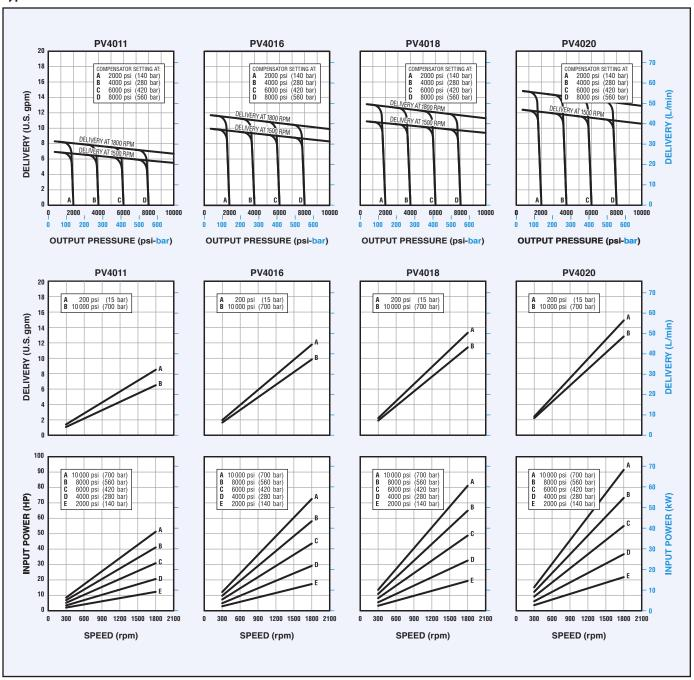
Typical performance curves are based on 100 SUS (20 cSt) mineral oil with pressurized inlet where required. Refer to "Minimum Inlet Pressure" table on page 2.
