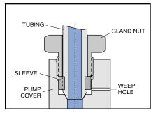
Typical Coned and Threaded port connection
