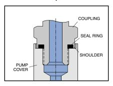
Typical British Standard Pipe (Parallel) port connection
