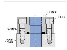
Typical SAE 4-Bolt Flange port connection
