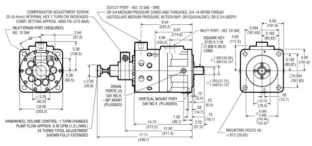
Handwheel Volume Control Model
